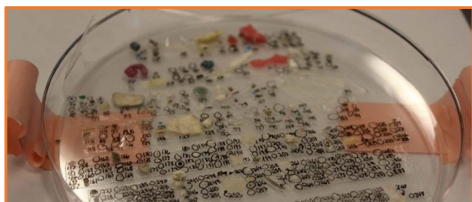
Example of a subset of microplastics collected from a single experiment. The large end of the MP scale is visible to the naked eye.
